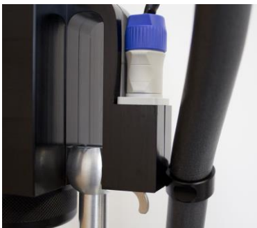
Fig. 16: Attaching the heated intake hose to the digital mass scale unit
