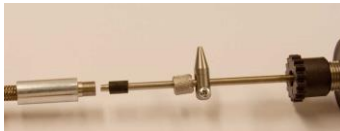
Fig. 67: Sampling probe removed from the intake hose
