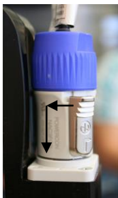
Fig. 88: Inserting the connector plug
