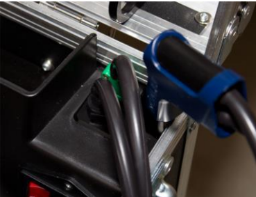
Fig. 39: Probe and cable-hose assembly connection for draft measurement
