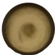
Fig. 10: Filter cartridge visibly loaded
