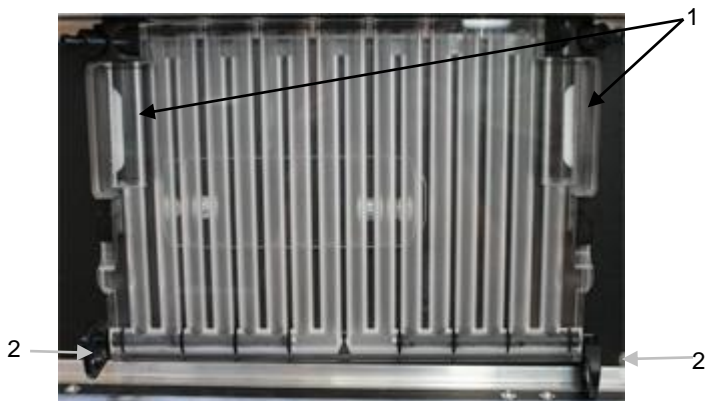
Fig. 62: Close-up view of the flue gas condenser
