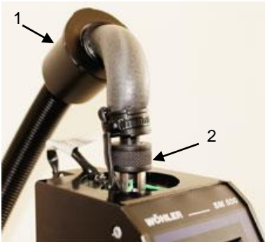
Fig. 84: Disconnecting the heated sample intake hose
