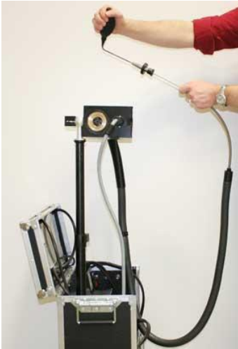
Fig. 72: Purging the sampling probe, the hose and the digital mass scale unit
