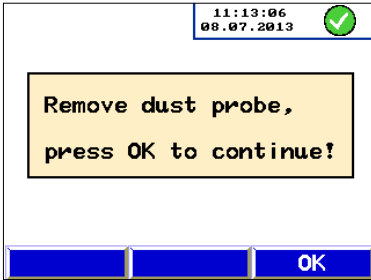
Fig. 31: Display immediately following the measurement
