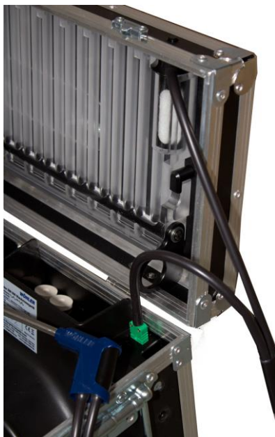
Fig. 13: Connection for flue gas analysis (special circumstances!)
