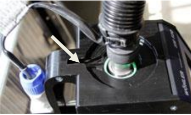
Fig. 89: Indentation for the connection cable of the heated sample intake hose
