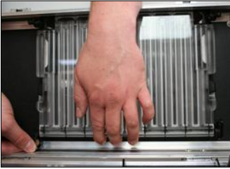
Fig. 65: Refitting the condenser
