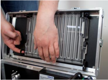
Fig. 63: Removing the flue gas condenser
