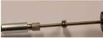
Fig. 71: Particulate-matter sampling probe connected to the heating hose
