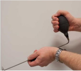
Fig. 73: Cleaning the sampling probe
