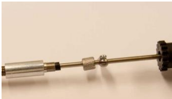
Fig. 75: Rubber seal inserted into the end piece of the heating hose
