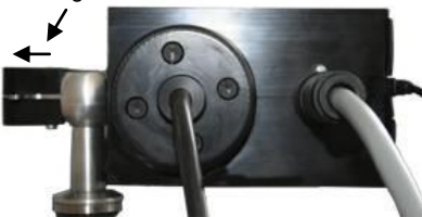
Fig. 5: Undo the locking latch on the digital mass scale unit
