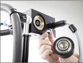
Fig. 68: Inserting a used filter cartridge
